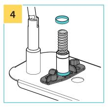
Slide portion ring over spring housing. Reassemble.
