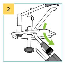
Pull down to separate pump body from lid assembly.
