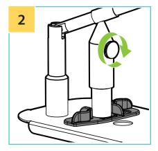
Secure the piston by tightening the thumb screw in the upper piston assembly.
