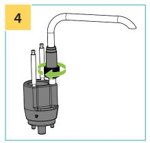
Screw the discharge tube assembly to the pump body.
