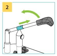
Slide collar up, lift handle clear of upper piston assembly.
