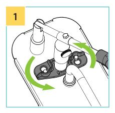
Twist lid lock counter-clockwise to unlock Lid.
