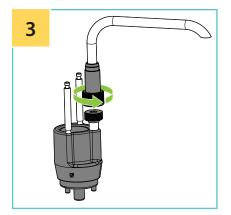
Unscrew the discharge tube assembly from the pump body.
