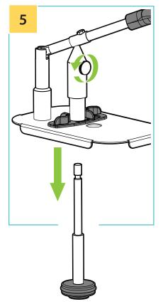
Loosen the thumb screw in the upper piston assembly. Pull the piston through the lid.
