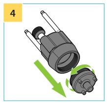
Unscrew the lower valve assembly from the pump body.
